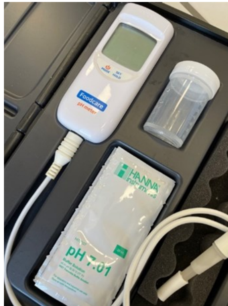
Figure 80 : pH-mètre Foodcare HANNA®instruments (Smart Gastronomy Lab, 2022)
