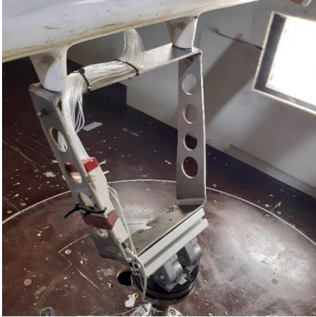
Figure 13. Wind tunnel pressure test set-up. Detail of the pressure tubes exit
