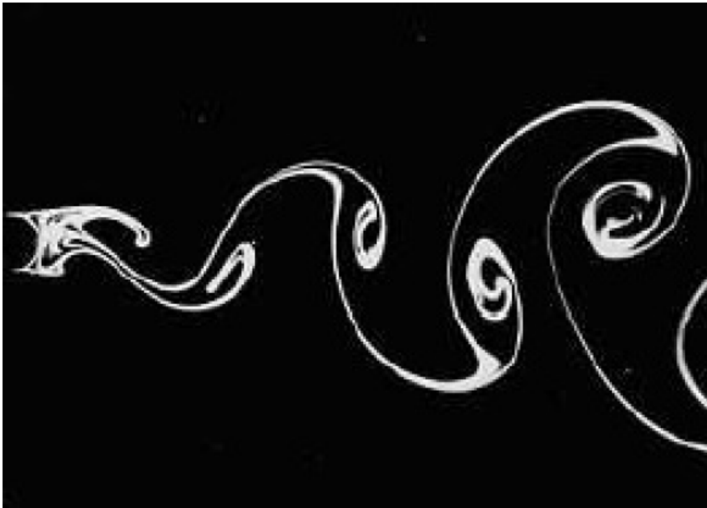
Figure 1.1: Example of a flow past a circular cylinder: formation of the Von Kármán vortex street at Re = 140 [61]
