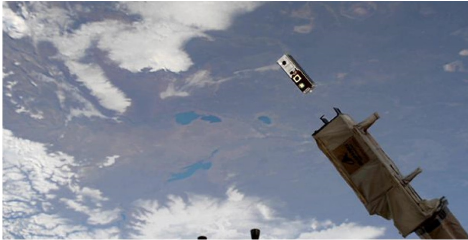
Figure 2.17: DeMi CubeSat deployed from the International Space Station on 13 July 2020 (image credit: NASA)
