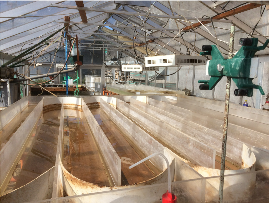
Figure 18: Small-scale HRAP ("basin 2") used to perform the tests of January 2020.
