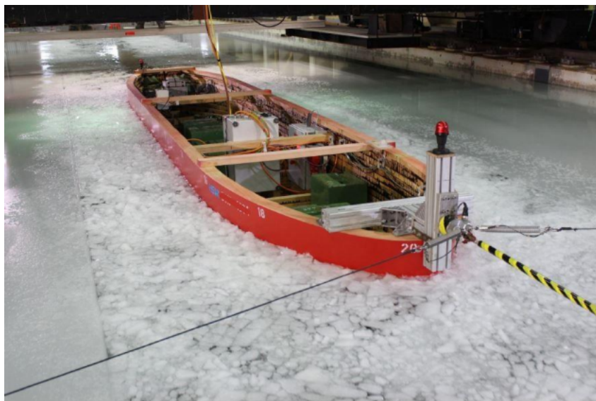
Figure 4: Brash ice model test at HSVA [4]
