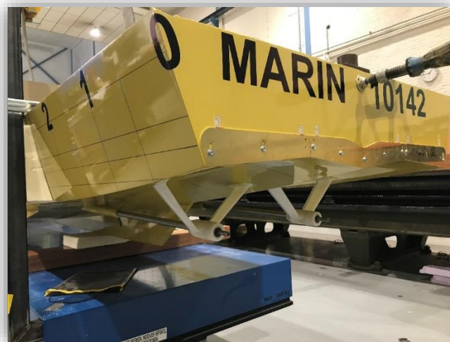
SHIP A model used for towing tank test
