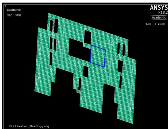
1 Panel failed after 3 rd iteration
