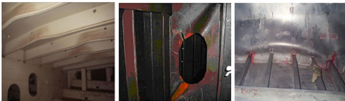
Figure 1. Local structural collapse/plastic buckling/damages in ship structures (DNVGL, 2015)
