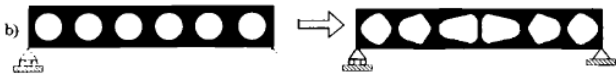
Figure 3 Shape Optimization (Bendsoe & Sigmund, 2003) Size Optimization
