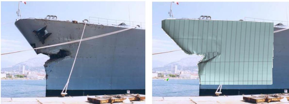
**Figure 43:** Comparison of LS-DYNA/MCOL simulation with real ship. (From: Le Sourne et al., 2003)
