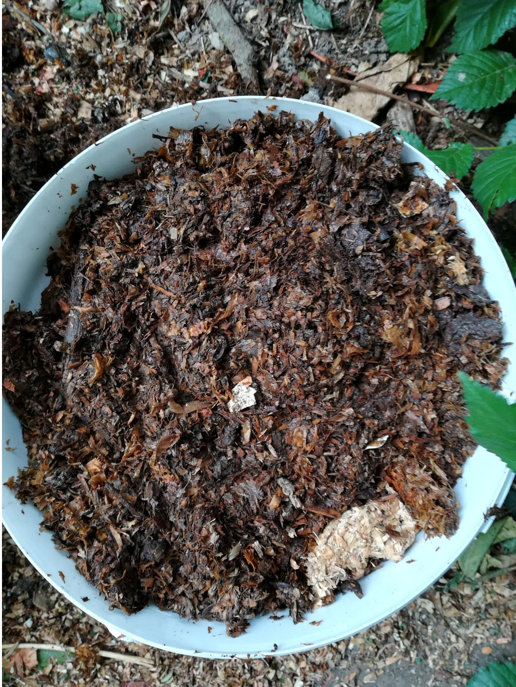
Figure 9 – KT6 sample : 6 months old kitchen waste and BLT material. Moisture content is higher than KT0.
