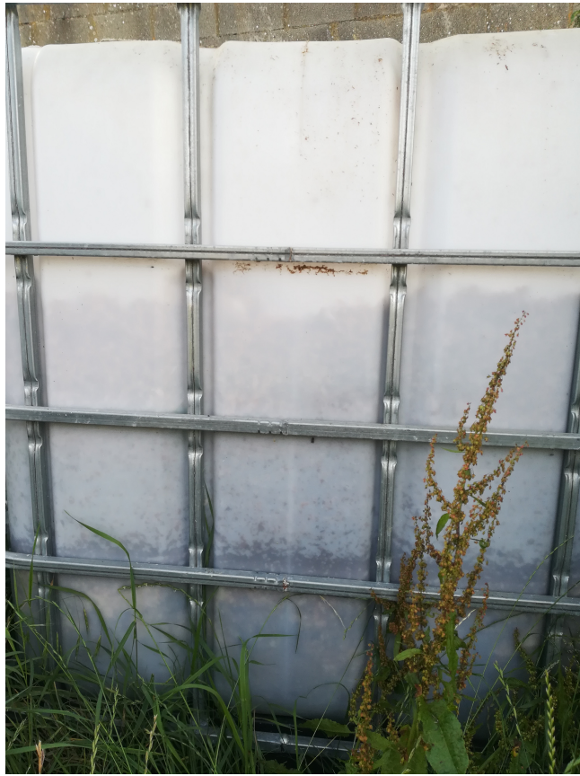
Figure 17 – Outside view of the bottom (T8-Bot) soaked in liquid due to waterproof floor, at the level of the metal bar. Upper part (T8-Top is moist but not soggy.
