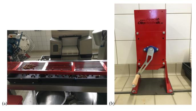
Figure 9 – (a) Calibration sieves and (b) hand cracker "WAL MAN" from Feucht-Obsttechnik.
