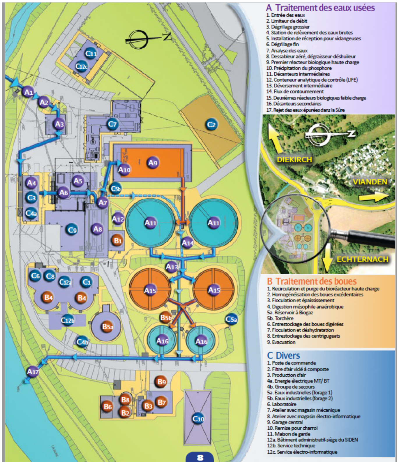
Figure 14: Detailed Illustration of the Blesbruck WWTP
