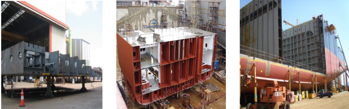
Figure 7. Semi-block, Block and Grand Block Assembly
