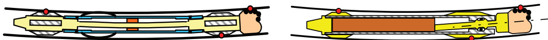
(a) Internally deflected driveshaft on a non-rotating housing (b) Geo-stationary unit keeps bit tilt angle in a rotating section
