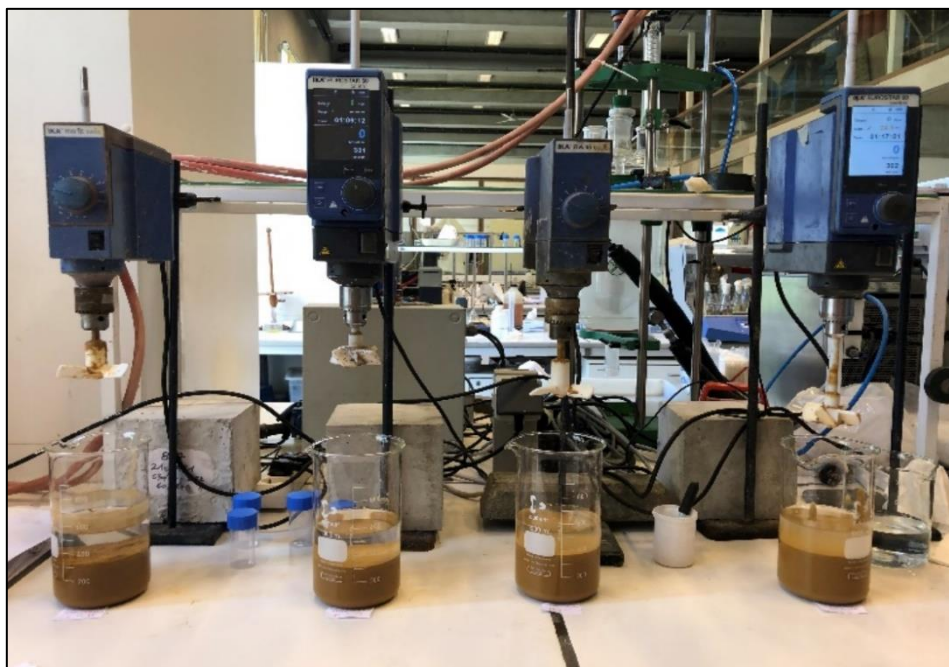
Figure 25: Jar test set-up used for pH optimization
