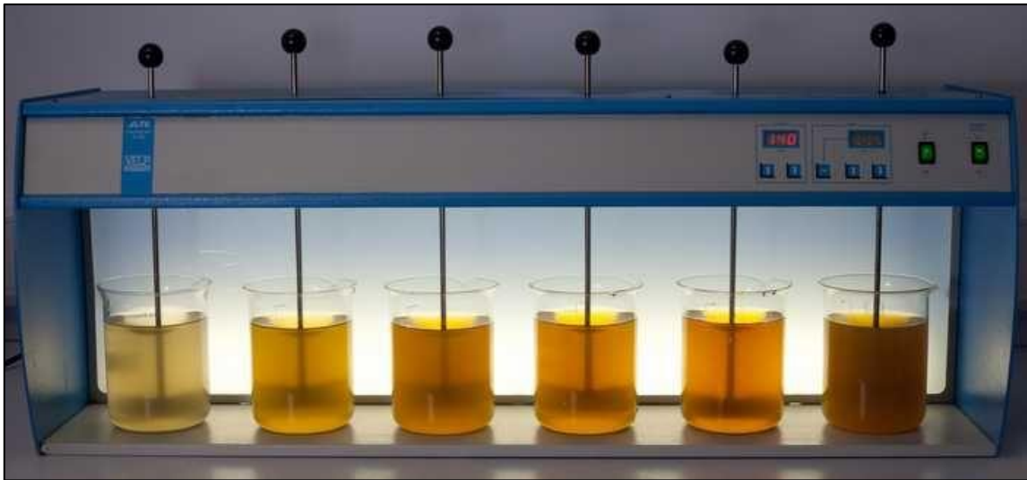
Figure 22: Standard jar test protocol
