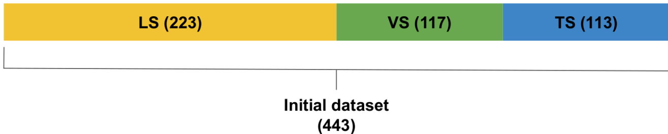
Figure 5.2: Illustration of the division of the initial dataset into 3 parts: the Learning Set (LS), the Validation Set (VS) and the Test Set (TS). The scalars in parentheses correspond to the number of multi-feature images contained inside each set.
