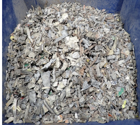
Figure 8.3: Illustration of the mix of scraps (called real test set) used to evaluate an estimation of the real performance of the final Mask R-CNN model: the objects have various shapes and the class distribution is completely unknown.
