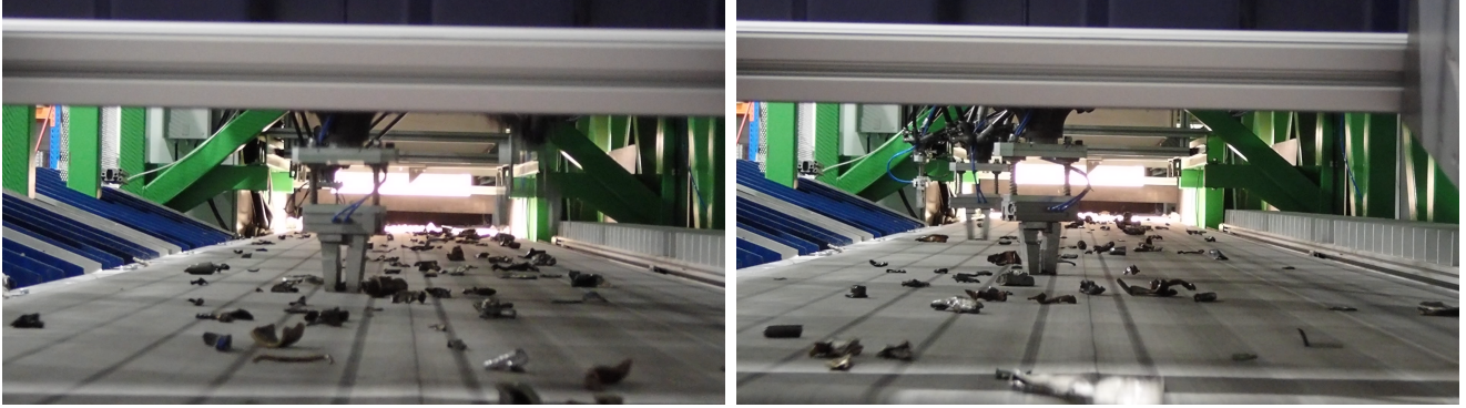
Figure 8.4: Illustration of the delta-robots grasping some scraps on the moving conveyor belt during the real assessment. We can observe that the conveyor belt is saturated with scraps.
