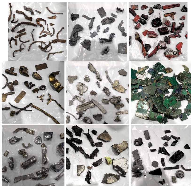
Figure 10.1: Overview of the 9 classes of scraps considered in this master's thesis. First row: copper, laminated zinc and paint samples. Second row: brass, aluminum, and PCB scraps. Third row: nickel, rubber and zamak objects.
