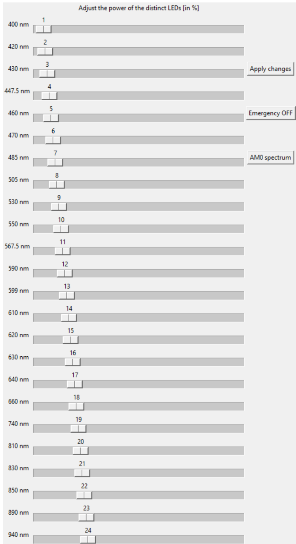
Figure 45 – Graphical interface of the calibration script.
