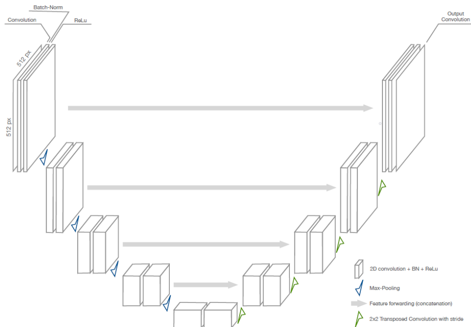
Figure 2.9: The FCNN architecture (Source: [Sakinis et al., 2019]).
