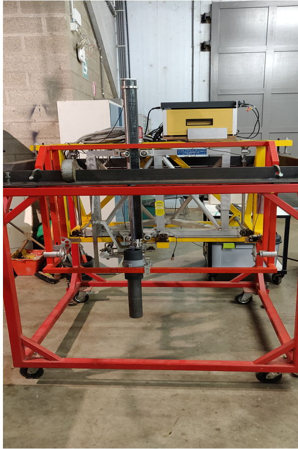
Figure 3.28: Balance used in the towing tank
