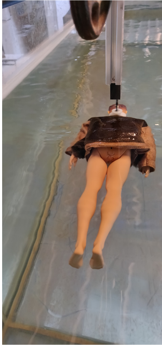
Figure 3.59: Parachute effect on the model
