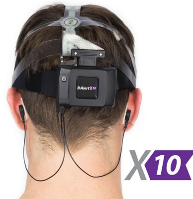
Figure 2.10: Mastoids illustration, fixing the gain of the channels of the 9 brain EEG sites.
