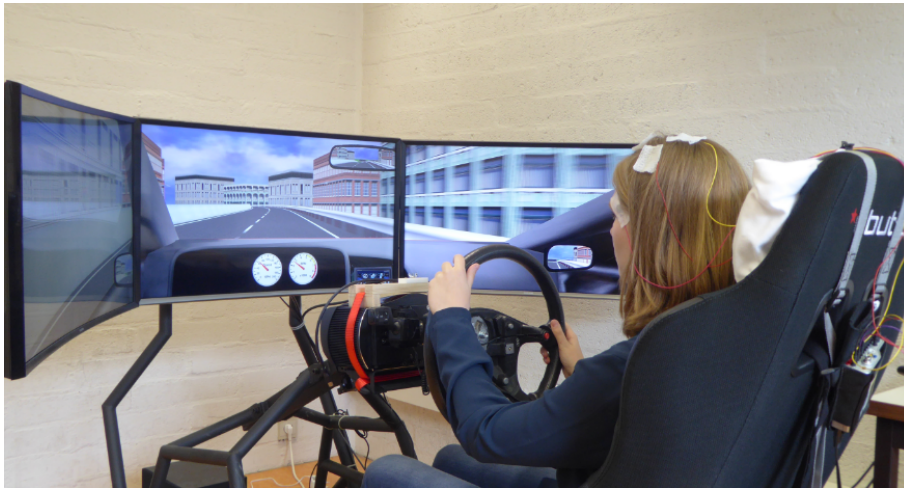
Figure 2.1: Fixed-base driving simulator at the University of Liège [44].
