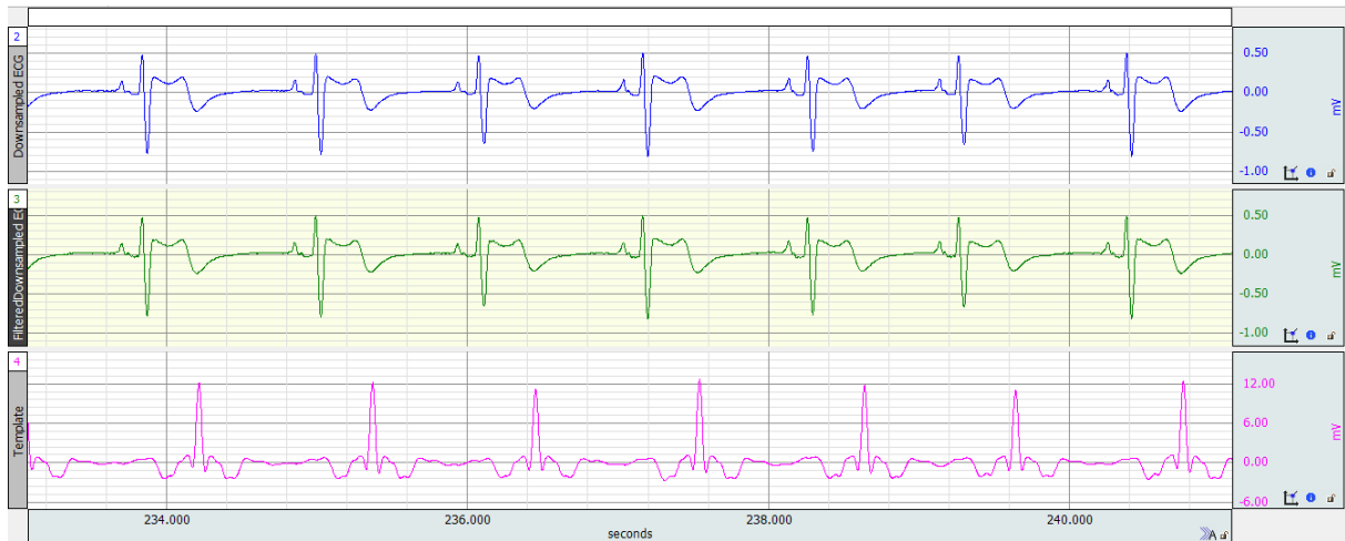
Figure 3.1: Examples of downsampled ECG (500 Hz), band-pass filtered ECG (0.5-35 Hz) and template signal obtained using AcqKnowledge .
