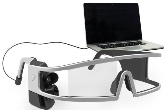
Figure 2.13: Phasya Glasses and laptop on which the Drowsilogic software is installed [44].
