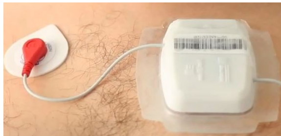
Figure 1: wearIT4Health prototype[7]: around 5 cm x 8 cm.
