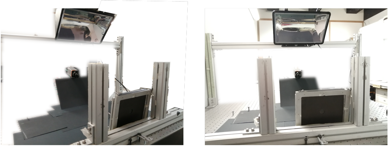
Figure 6.5: Experimental set-up in thermography. Example with the sample \text{FBH}_{\text{clamped}} .
