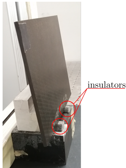
Figure 6.6: Set-up of sample \text{FBH}_{\text{free}} and 3, sample \text{FBH}_{\text{free}} is shown but the same set-up is used for the sample POR.
