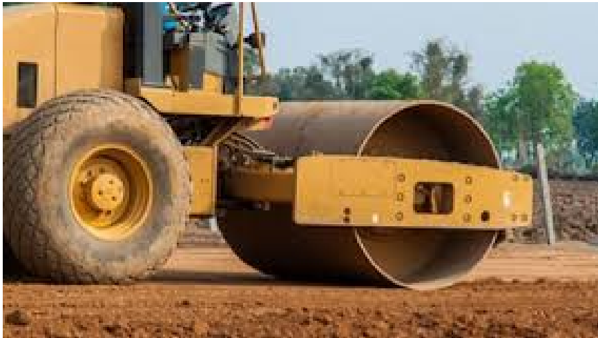
FIGURE 9 – Machine de compaction par impact à rouleau [ https://leica-geosystems.com/fr-be/products/total-stations/software/leica-captivate/expert-insight-compaction ]
