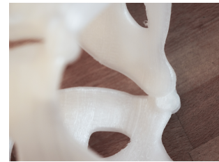
(c) Merged parts due to insufficient gap between the upper arm and the forearm parts when printed in a V-shape.
