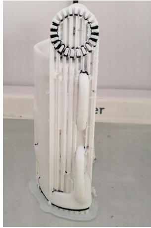
(a) Blocking hinge printed vertically in PET, supports in PLA were added.
