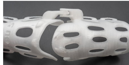
Figure 22: Trial of design simplification using only one hinge. Note that the hinge design is the initial one and is thus very bulky.
