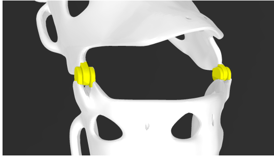
(a) Initial free hinge used in the BOA design. To be embedded in both parts of the splint and to print in one piece. The gaps inside the hinge were made to avoid merging of the articulation. No external piece is needed but the piece is more fragile.
