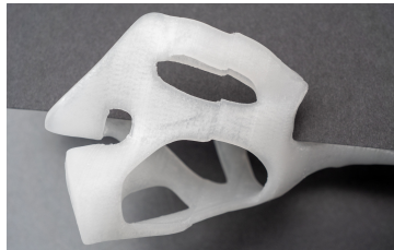
Figure 27: Piece with shifted layers. Note that on this model the shift is small does not impact too much the quality of the piece, at least for prototyping.
