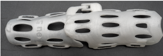
Figure 22: Trial of design simplification using only one hinge. Note that the hinge design is the initial one and is thus very bulky.
