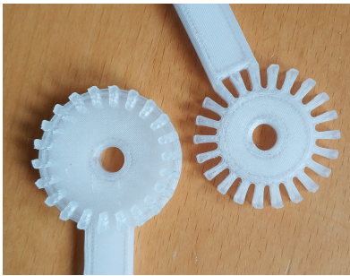
(a) Blocking hinge printed horizontally in PP, no supports were needed. Very good result, the parts are precise and fit perfectly
