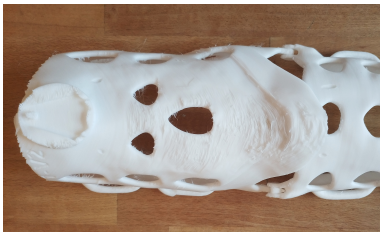
(a) Bad finishing quality due to supports on the outer surface of the splint.
