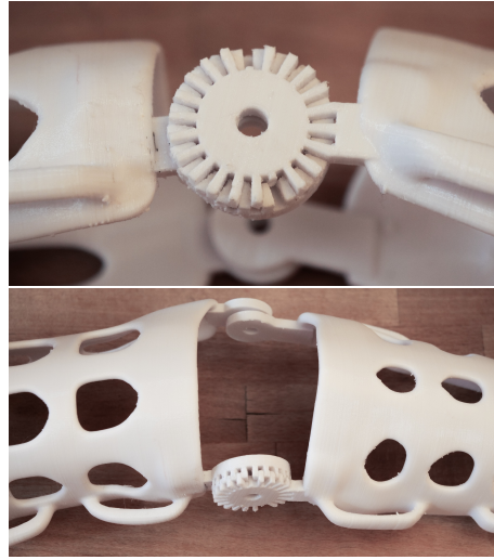
(b) Blocking hinges printed vertically in PET. Supports in PLA were removed. The missing teeth are noticeable and the two parts do not fit easily.
