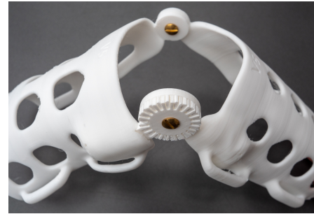
(b) Prototype using hinges clipped into the splint.
