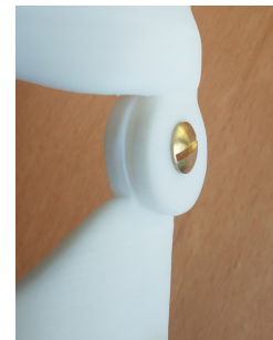
(b) Free hinge. One part is embedded in the upper part of the splint and the other one is embedded in the forearm part. They are secured by a binding screw.
