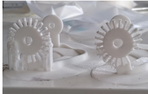
(b) Blocking hinges printed vertically in PP. Supports in PP were added on the hinge on the left but they cannot be easily removed and the quality is mediocre. The hinge on the right was printed without any supports, some teeth are missing and the quality is also very poor. Both parts are unsatisfying.
