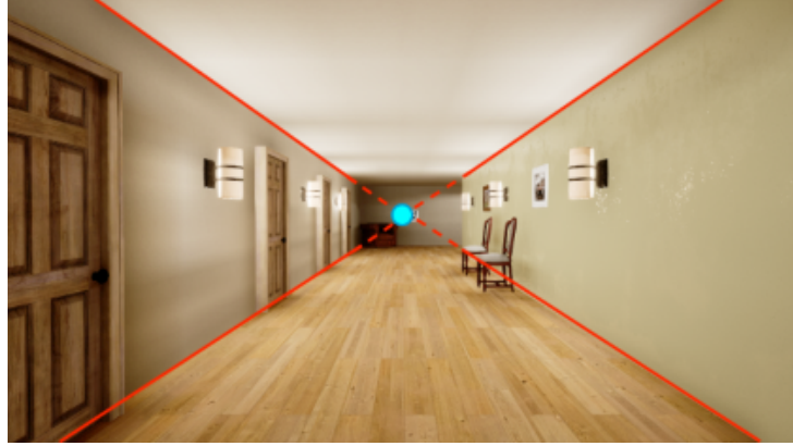
Figure 6.2: Example of a vanishing point (in blue) in a corridor image. The parallel lines (in the real world) are represented in red.
