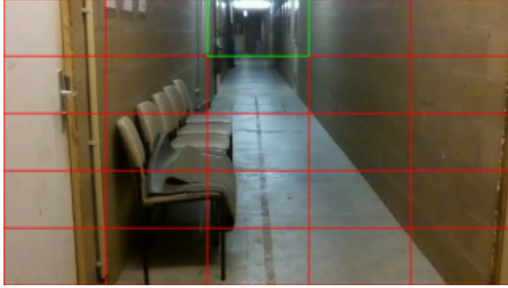
Figure 7.3: Example of a vanishing point detected via the VPDeepLearning method on a real world image.
