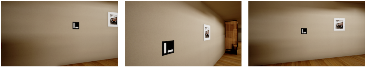
Figure 6.14: Examples of images collected for the evaluation of the ArUco marker detection and decoding method.
