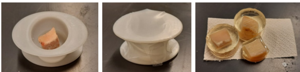
Figure 2.2: Illustration of the embedding process of samples. From left to right : cylindrical mold with sample inside, paraffin and embedded samples obtained.
