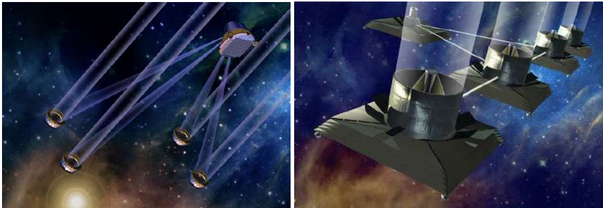
(a) Square configuration with remote communication and light path. (b) Linear configuration with physical link between telescopes.
