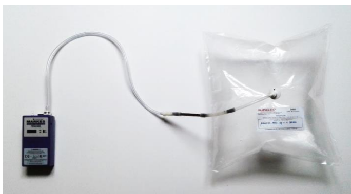
Figure 4: Concentration of the exhaled breath, contained into a Tedlar® bag, onto a TD tube
