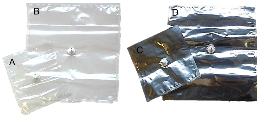
Figure 20: The four bags tested for the benchmarking study: (A) classic Tedlar® bag of 1 L, (B) classic Tedlar® bag of 5 L, (C) multifoil bag of 1 L and (D) multifoil bag of 5 L
