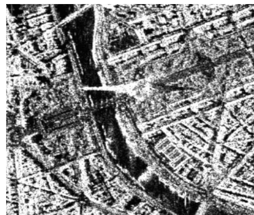
Figure 2.8: Layover effect. Layover is a special case of foreshortening. Top of a tall elements of the scene is closer to the sensor than the bottom. Following the rule that image is constructed in range with the distance, the top appears first in the sensor direction. The right image illustrates layover with the Eiffel tower that seems to be laying on the side.
