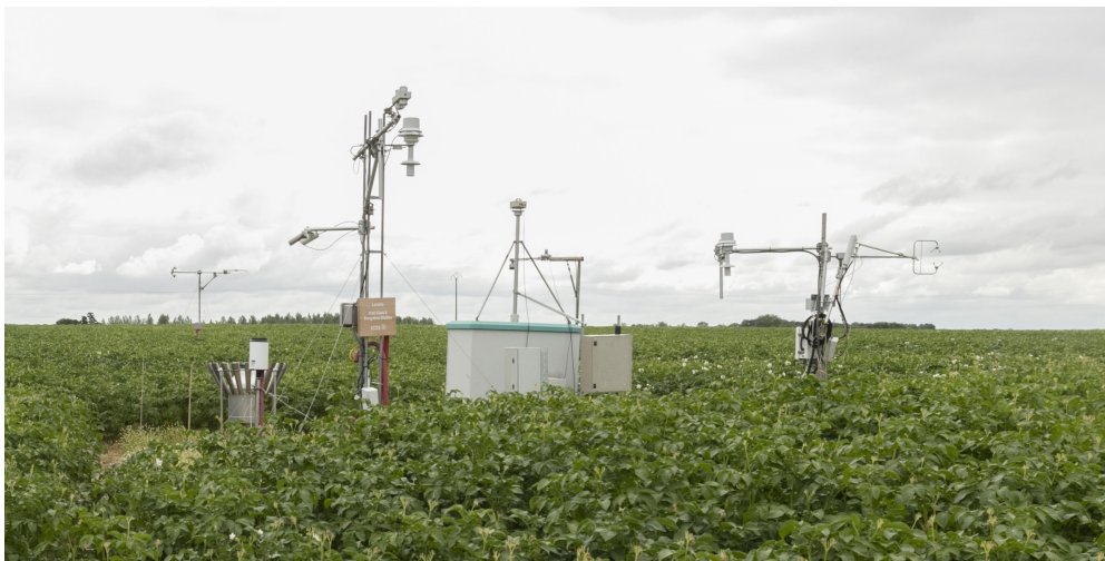
Figure 7: EC acquisition system and weather station in the Lonzée ICOS experimental field
