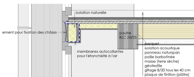
Figure 35 – Raccord de plancher 2
