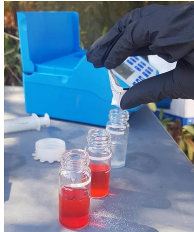
Figure 23: Cuvette with all the nitrite reagents becoming red (concentration of 43\mu\text{g/L} ).
