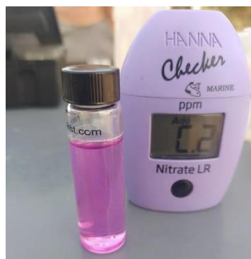
Figure 21: Cuvette with all the nitrate reagents becoming pink (concentration of 0,3 PPM) and the checker.
