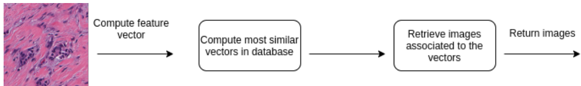
Figure 3.2: Overview of the second methodology. The retrieved images are to the nearest feature vectors of the query image feature vector.
