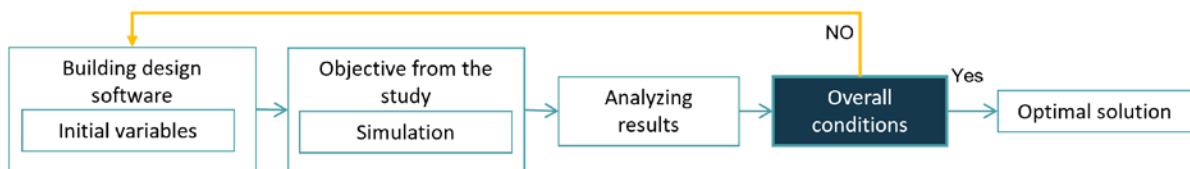
Figure 4-4 Workflow parametric design based on building performance
