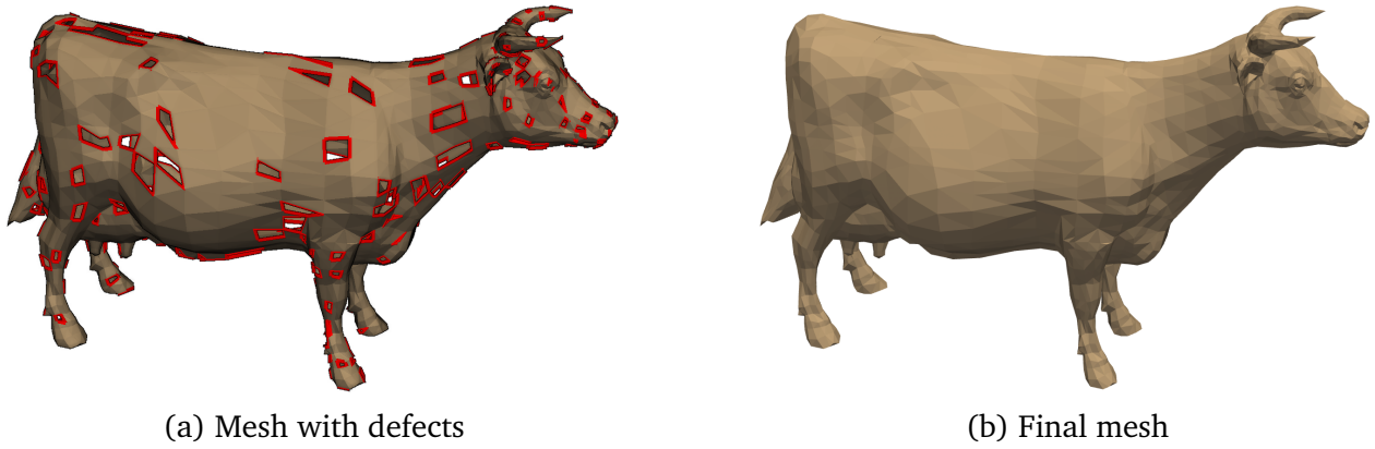
Figure II.7: Mesh fixing using pymeshfix .
