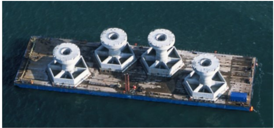
Figure 15. Shallow water concept: Nysted I offshore wind farm foundations [13]
