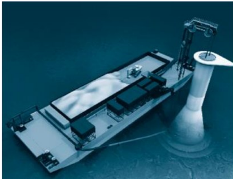
Figure 12. Multi-purpose barge Thornton I depicted in permanent ballasting and backfilling [11]
