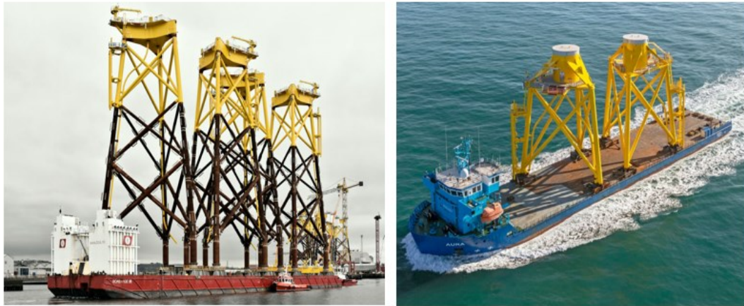
Figure 21. Transportation of jacket structure from land [19]
