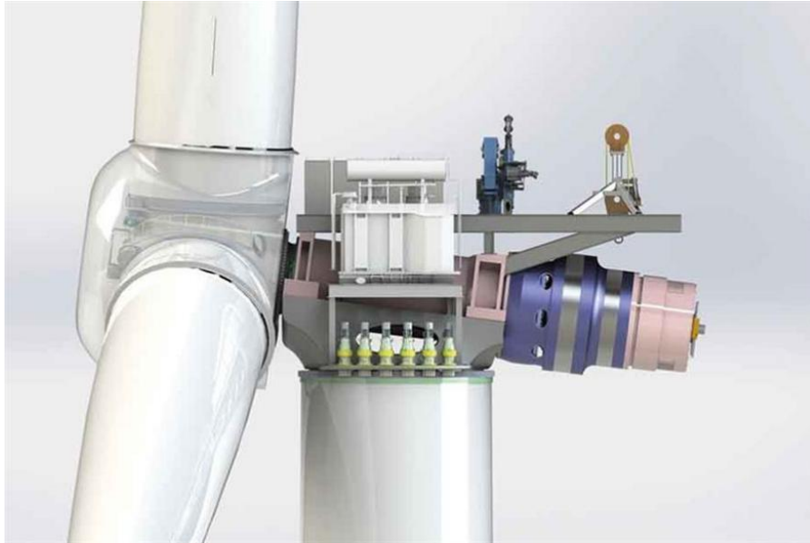
Figure 4: Generator system of FWOT (Source: windpowermonthly.com)
