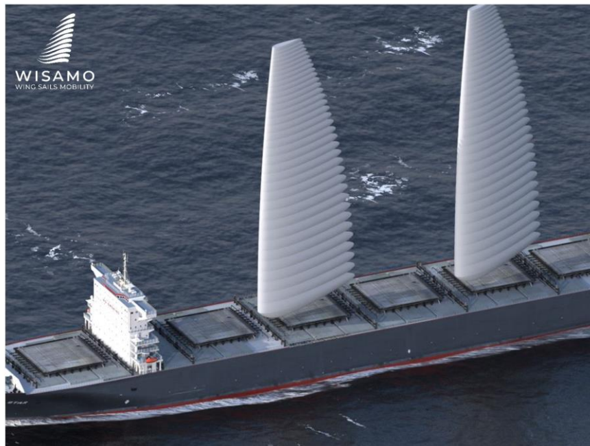
Figure 12 – WISAMO inflatable sails (Michelin, 2021)
