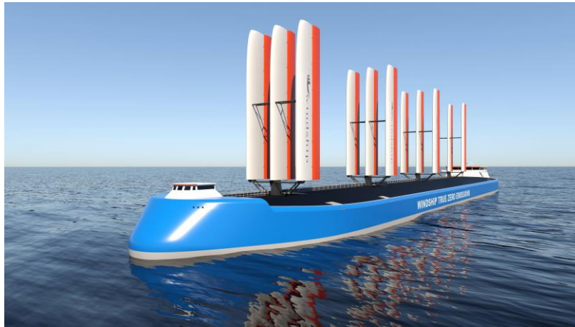
Figure 9 – Windship Technology rigid wing sails (Ovcina, 2021)
