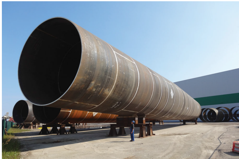
Figure 2.6: A 7.5 m diameter monopile for GodeWind OffshoreWind Farm [19].
