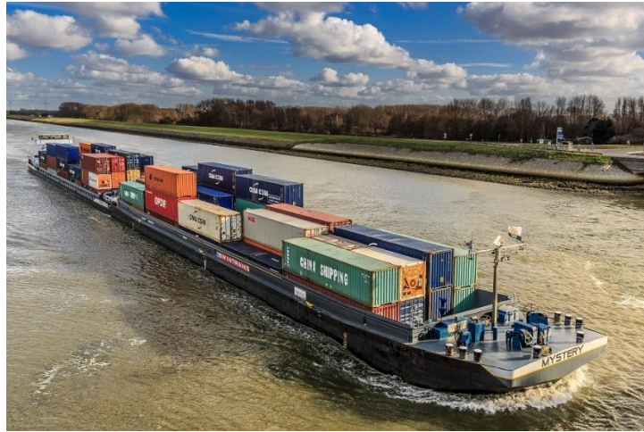
Figure 5: Coupled formation: Company; L: 94.90m - B: 11.45m – D: 3.65m-T: 2765/160TEU Barge Mystery; L: 76.46m - B: 11.43m – D: 3.85m -T: 2665/160TEU. Available from http://www.daribv.com/en/our-fleet/freighters/company-mystery [Accessed 12 Jul 2021]
