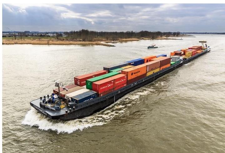
Figure 4: Coupled formation: Contargo1; L: 97.55m - B: 11.40m – D: 3.51m-T: 2848/176TEU Contargo X; L: 83.10m - B: 11.45m – D: 3.67m -T: 2673/172TEU Available from http://www.daribv.com/en/our-fleet/freighters/contargo-i-contargo-x [Accessed 12 Jul 2021]
