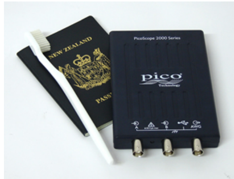
Figure 2.3: Picoscope 2000 series. Dimensions (including connectors) are: 142 x 92 x 18.8 mm.
