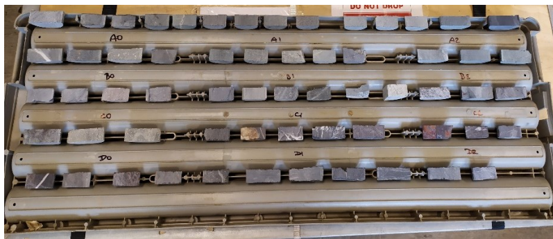
Figure 33. Rock pieces sliced from the main drill-core samples (prepared for XRF scanning)
