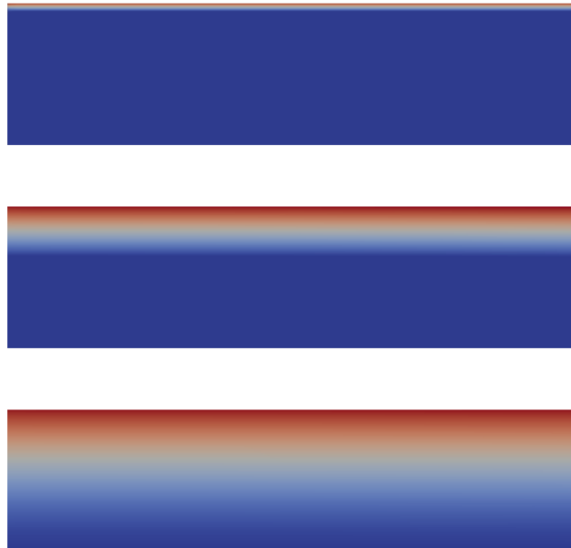
Figure 3.6: Time evolution of natural corrosion diffusion
