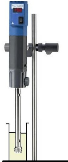
Figure 56: Rotor Stator Homogenization [29]
