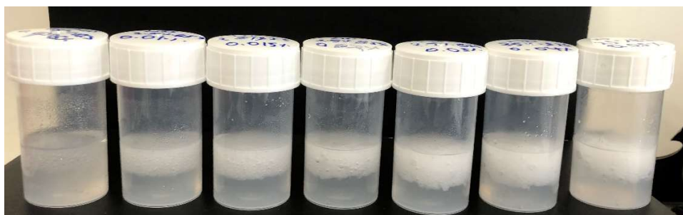
Figure 53: Macroscopic Images of emulsions prepared by 2.5% BIS large microgels using large axis and PDMS
