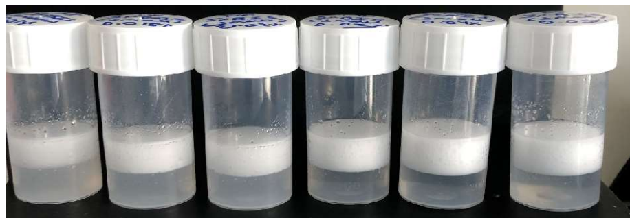
Figure 54: Macroscopic Images of emulsions prepared by 2.5% BIS small microgels using large axis and PDMS
