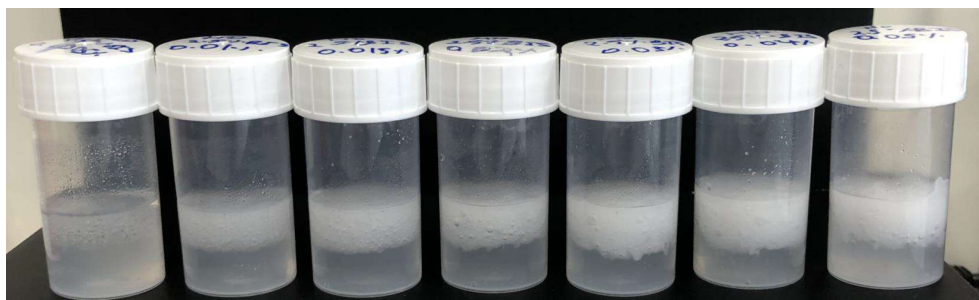
Figure 52: Macroscopic Images of emulsions prepared by 1% BIS large microgels using large axis and PDMS
