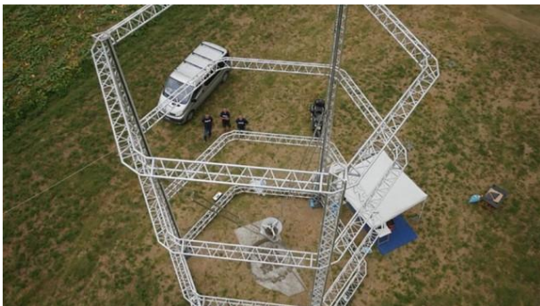
Figure 74 : WASP, Imprimante 3D Big Delta, Italie, 2015.
