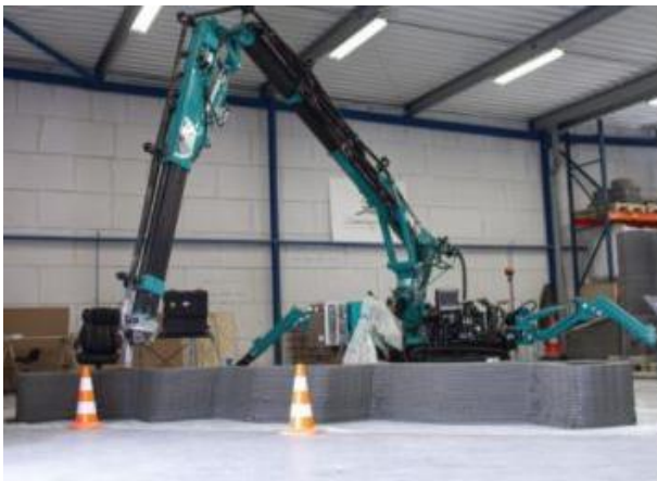
Figure 72 : Constructions-3D, Imprimante 3D MAXI PRINTER, France, 2017.
