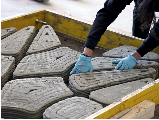
Figure 33 : Team DBT, formwork, ETH Zurich, 2021.
