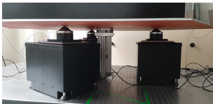
Figure 26: Picture of the three isolators. A sphere is used to have the smallest contact point between the isolators and the hexagonal table. The guide in the center is not in contact with the hexagonal table. It is only placed there for safety reasons in case of an accident.
