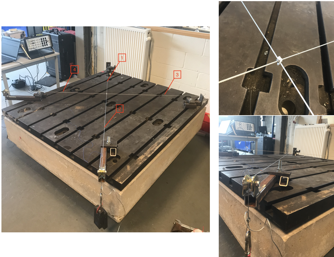
Figure 3.7: Assembly of the cross-cables network set-up
