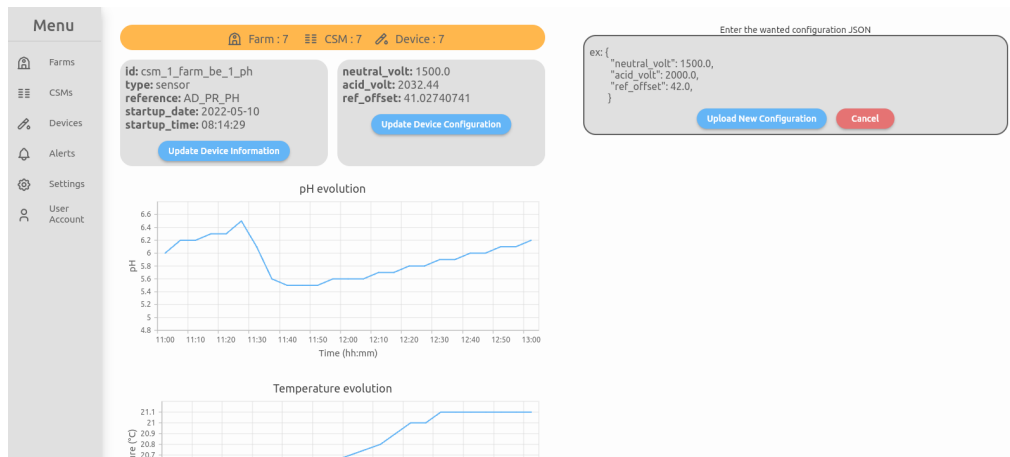
Figure 6.14: The desktop version of the update configuration page (UpdateBody) of the device view of the MD.
