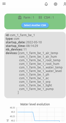
Figure 6.11: The smartphone version of the CSMs detailed page (CsmPageBody) of the CSM view of the MD.
