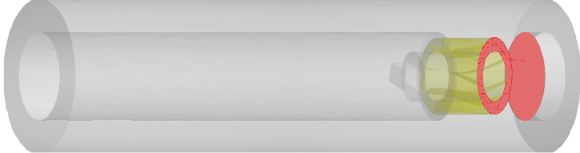
Figure 4.4: Acoustic set-up with Lighthill surfaces in red and Lighthill volume in green.
